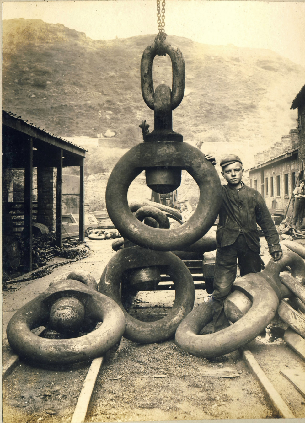
6" Iron—Test 140 Tons Tensile Strain.
